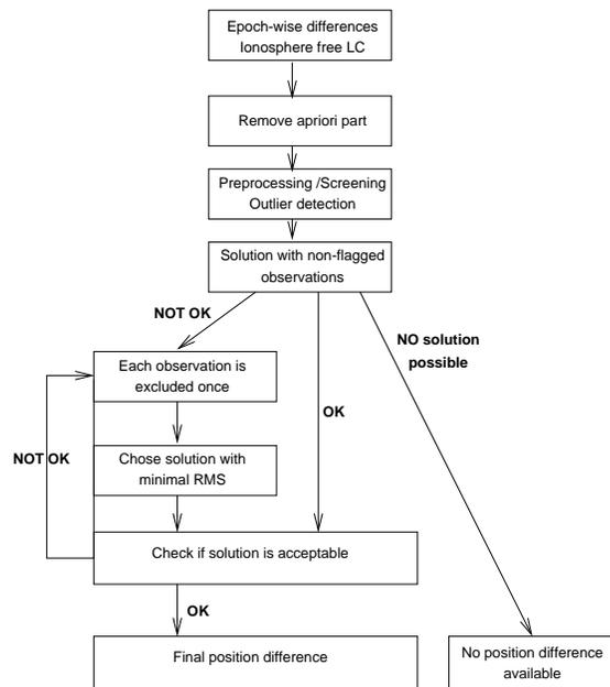
**Fig. 2** Processing scheme for deriving position differences from the phase
