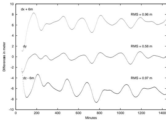
**Fig. 4** Differences between CHAMP - RSO and dynamic orbit accelerometer data used, **D5** is input - 01/152.
