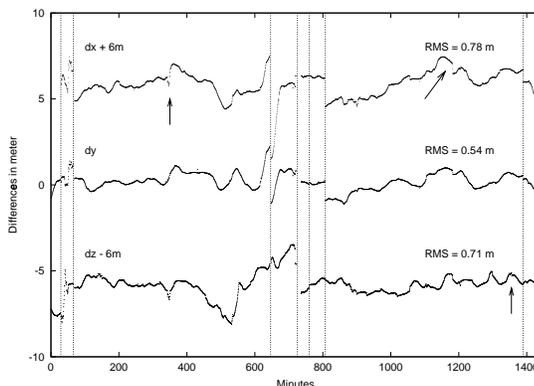
**Fig. 3** Differences between CHAMP - RSO and kinematic orbit **D5** - 01/152.
