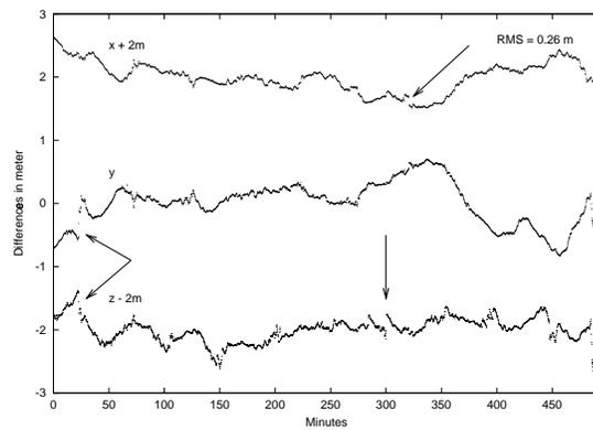
**Fig. 1** Differences in  $x, y, z$  between kinematic and dynamic orbit for SAC-C on 01/051. Arrows indicate jumps in the kinematic solution.
