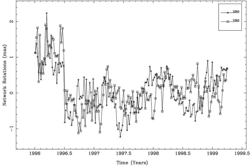
Figure 2: Effect of reference frame changes (IGS orbits) on regional GPS network solutions (X- and Y-rotations).
